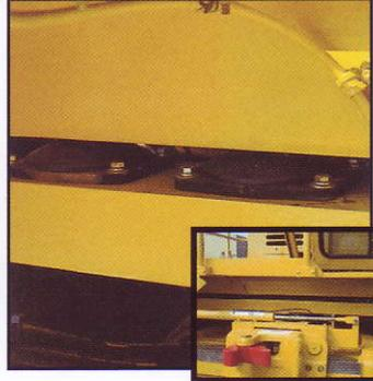
Rubber suspended body frame mounts = smoother ride and reduced operator fatigue.
