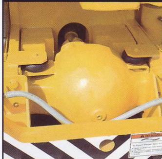
Meritor design axle = increased load capacity & mechanical differential lock.
