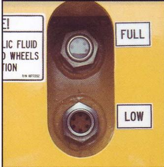
Hydraulic tank fluid level gauge = rapid maintenance checks
