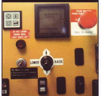
Combines six (6) separate displays into one (1) = single gauge focal point.
