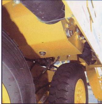
50 gallon hydraulic tank = additional cooling capacity for hydraulic oil.
