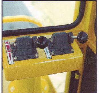
Rear brake/throttle hand controls = convenient operation from the rear operating position.
