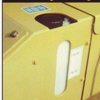
Radiator coolant level sight gauge = visual service checks.
