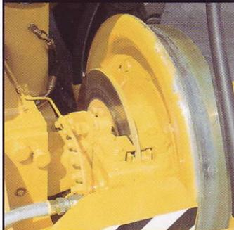
Meritor brakes with large caliper and discs = excellent braking and service characteristics.
